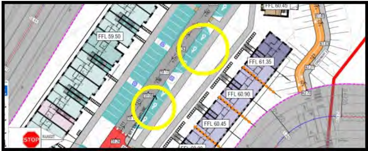
Figure 7 – Poor distribution of disabled parking spaces, and not 5% of total
