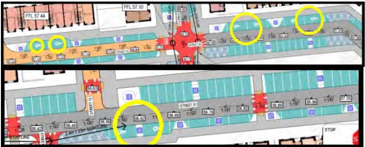
Figure 8 – No dropped kerbs shown at any disabled parking spaces in the development
